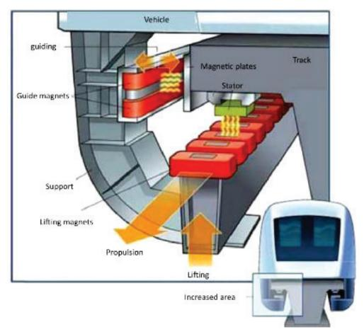
Fig. 11. EMS system used in Transrapid [6]
