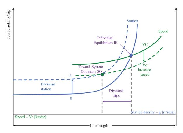
Fig. 4. Operation strategy for shifting individual equilibrium to system optimum
