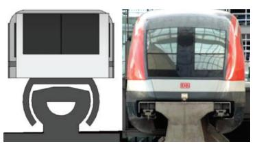
Fig. 29. Comparison between the proposed system 1 (ProDynamic) and the Transrapid system
