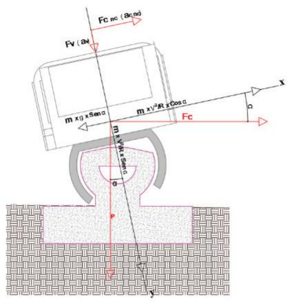
Fig. 35. Schematic of the forces acting (acceletarion directions) on the vehicle
