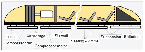
Fig. 4. Simplified scheme of "Hyperloop Passenger Capsule" [12]
