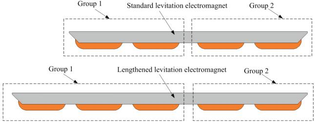
Fig. 8. Comparison of lengthened levitation electromagnets and standard levitation electromagnets
