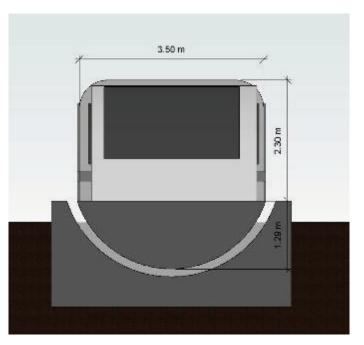
Fig. 42. Transverse perspective of system 2 vehicle
