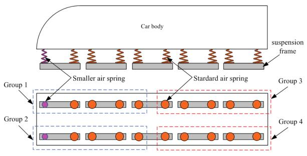
Fig. 6. Arrangement of air springs on the maglev train
