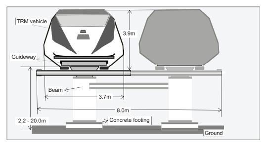
Fig. 2. Scheme of the right-of-way of the TRM system [1]
