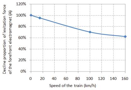
Fig. 5. Relationship between speed and levitation force of forefront electromagnet
