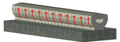
Fig. 24. Longitudinal scheme of the rail and the induced magnetic field, to generate the rotation
