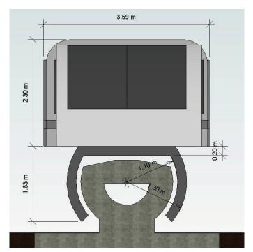
Fig. 32. Transversal perspective of the system 1 vehicle
