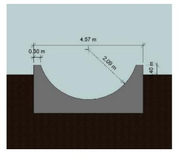
Fig. 41. Cross section of the proposed system 2 rail
