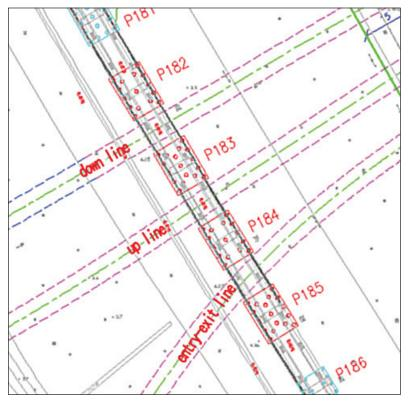
Fig. 1. Metro line13 traversing the maglev plane
