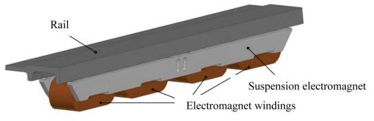
Fig. 3. Structure of rail and levitation electromagnet
