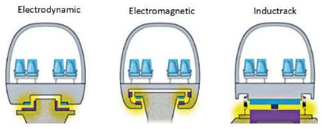
Fig. 20. Comparison systems between Magnetic Levitation Systems (Source: Maglev Trains A Look into Economic Concessions, Binyam Abeye, 2011)
