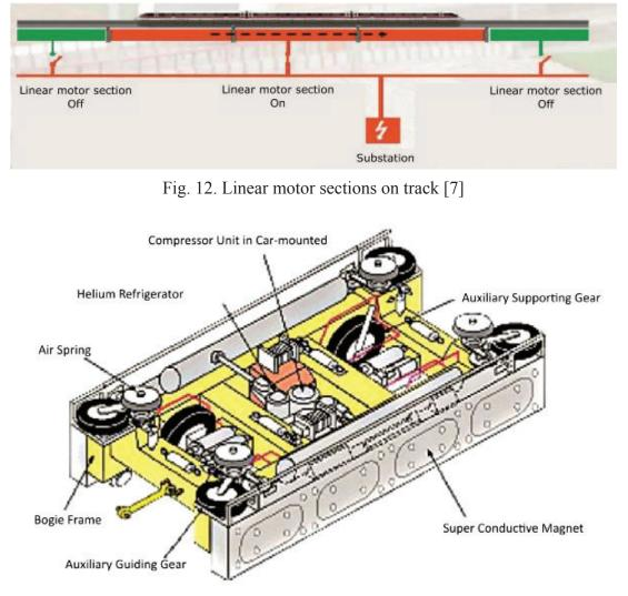
Fig. 13. MXL01 bogie system (Source: Odec.ca, HBLee, 2007)
