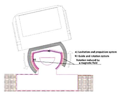
Fig. 23. Rotation scheme of the vehicle induced by a magnetic field
