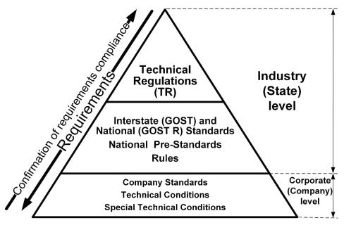
Fig. 2. The Russian system of normative technical regulation for safety
