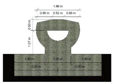
Fig. 31. Cross section of the proposed system 1 rail
