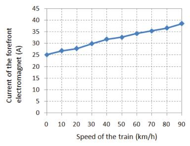
Fig. 2. Data of electromagnet current at different speeds of maglev train
