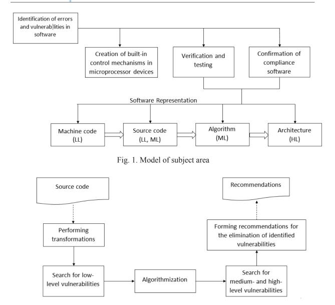
Fig. 2. Algorithm for creating error-free and impact-resistant software
