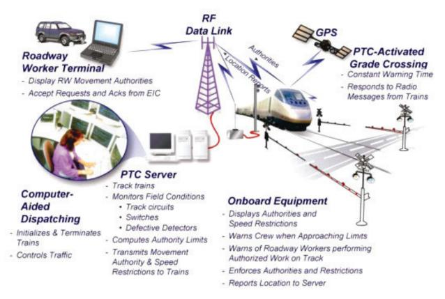
Fig. 2. Positive Train Control System Architecture [4]
