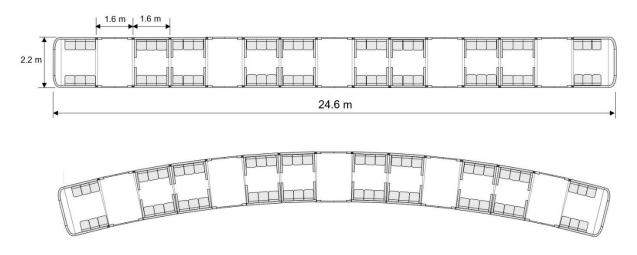
Fig. 3. Modular vehicle layout
