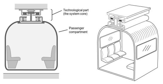
Fig. 1. The suspended Maglev configuration
