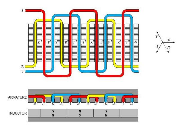
Fig. 7. The Linear Synchronous Motor (LSM)
