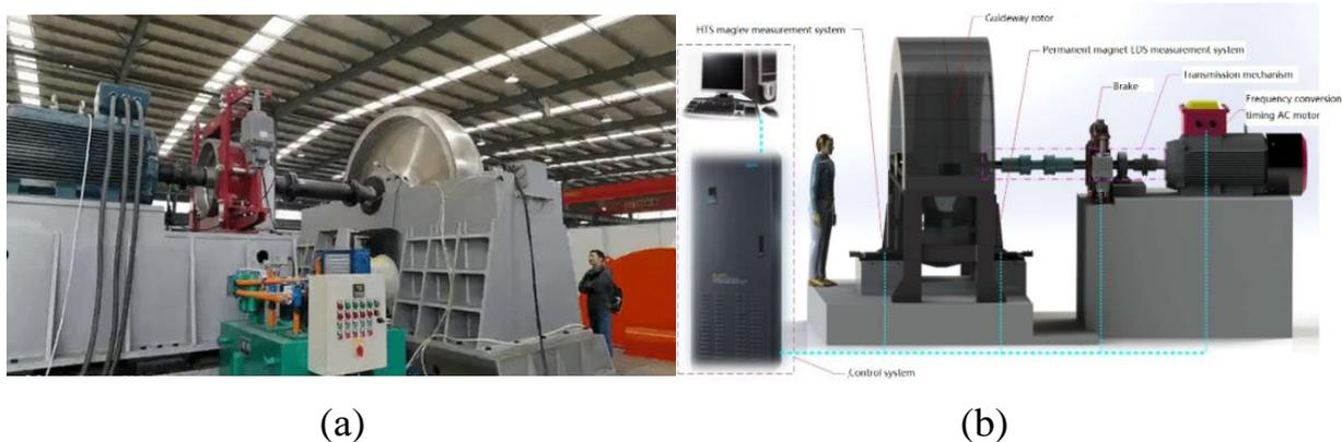
Fig. 10. The (a) photo and (b) schematic diagram of the rotating High-speed Test-Platform
